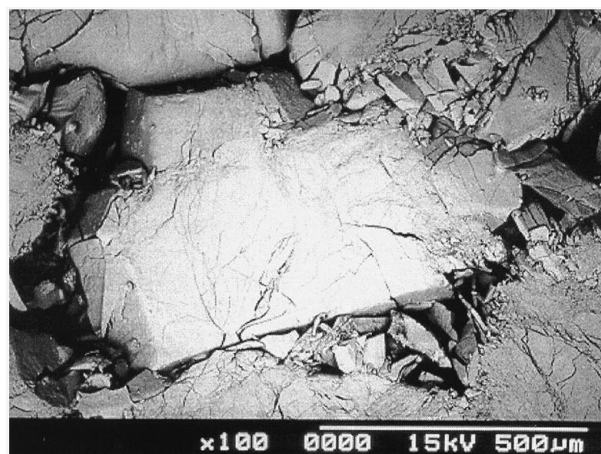
Figure 2. Photomicrograph showing cracks in sucrose crystals below 500 \mu\text{m} in diameter.
